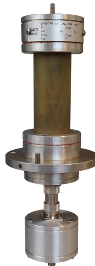
Fig. 14 Photograph of the INRIM divider in its final stage
