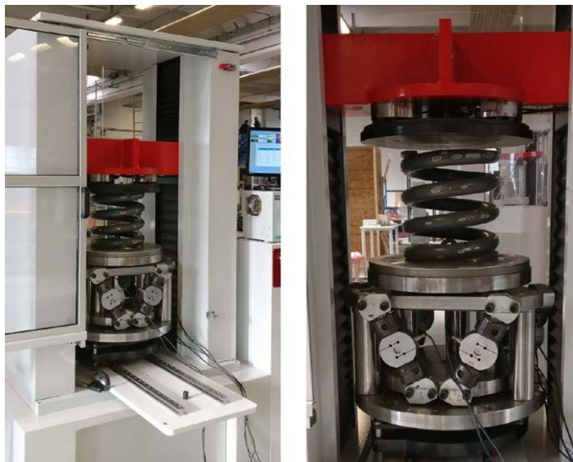
Figure 3. The 400 kN HS MFT integrated in the Easydur Aura Chasse railway spring testing machine.
