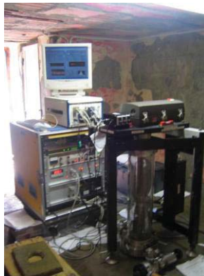
Fig. 1-2 - Gravity station at Serra La Nave (SLN, Mt. Etna): on the left the FG5#238, on the right the IMGC-02 during the measurements.
