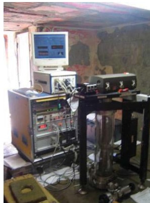
Fig. 2 - Gravity station at Serra La Nave (SLN, Mt. Etna): on the left the FG5#238, on the right the IMGC-02 during the measurements.
