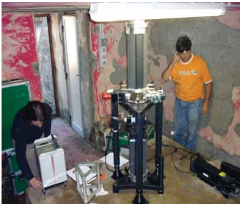
Fig. 1-2 - Gravity station at Serra La Nave (SLN, Mt. Etna): on the left the FG5#238, on the right the IMGC-02 during the measurements.
