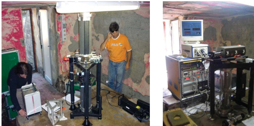
370 371 372 Fig. 2 – Gravity station at Serra La Nave (SLN, Mt. Etna): on the left the FG5#238, on the right the 373 IMGC-02 during the measurements.
