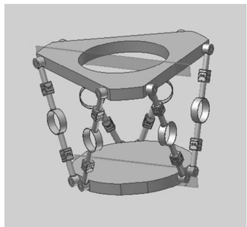
Fig. 3. Layout of the hexapod-shaped Multicomponent Force Transducer (MFT).
