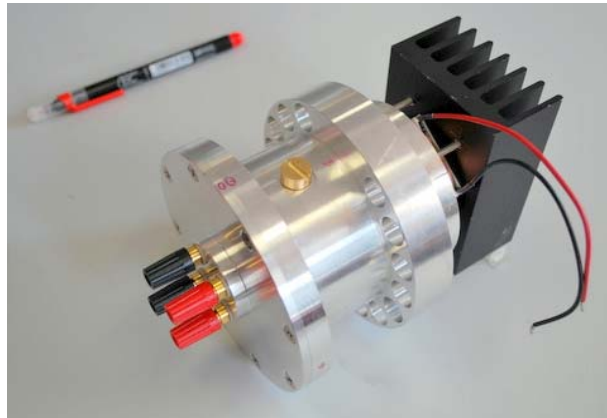
Fig. 1. View of the aluminium structure connected to a TEC and a heat sink.
