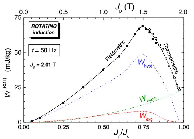
Fig. 4. Behaviour, at 50 Hz, of the rotational loss  $W^{(ROT)}$  and its components. It is remarkable the drop of  $W^{(ROT)}$  (solid line) onto its classical component (dashed line, Eq. (2)) at  $J_p \approx 1.96 \text{ T} \approx 0.98 J_s$ , and the corresponding vanishing of  $W_{hyst}^{(ROT)}$  and  $W_{exc}^{(ROT)}$ .
