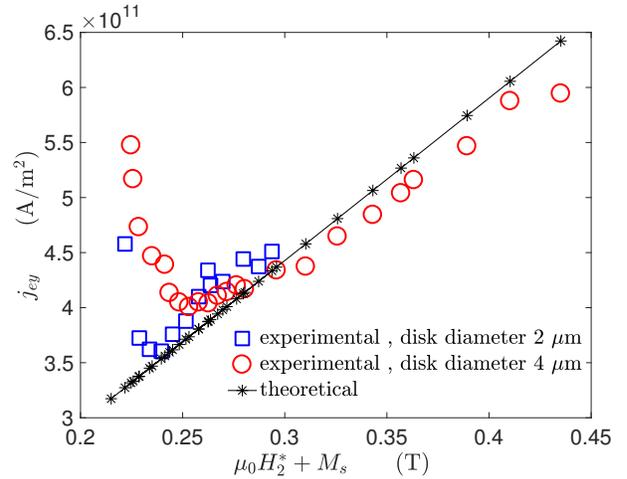
Figure 2: Threshold electric current density  $j_{ey}$  of Pt corresponding to the onset of self oscillations in YIG due to the spin orbit torque effect. Points: experimental data after Ref.[2] on YIG disks (20 nm thickness,  $2\mu\text{m}$  and  $4\mu\text{m}$  diameters). Line: theory, Eq.(14) with parameters given in the text. The magnetic field is  $H = H_{a,z} + M_s$
