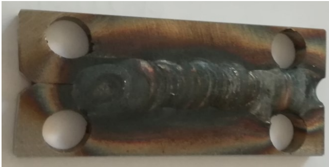
Fig.4. AISI sample welded by TIG
