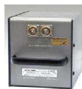
Fig. 5. 1 nF ESI SC1000 standard capacitor.
