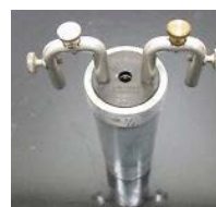
Fig. 3. 10 \Omega Leeds and Northrup 4030-B standard resistor.
