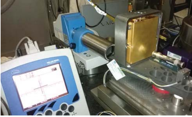
Fig. 10. Calibration of the accelerometer with the sine-bar nano angle generator (NAG). At the right side the nano angle generator with, on top of it, an accelerometer under test (golden box). In the background the autocollimator (AC) aiming at a mirror fixed to the NAG. Left front: the display of the AC.
