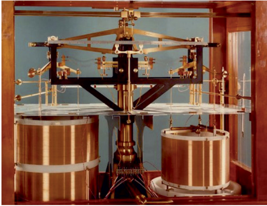
Figure 1: The ampere balance of the National Physical Laboratory. The balance has a symmetric design, with two fixed large solenoids and two movable suspended ones; one large coil has been removed to show the inner one. After more than 60 years of refinements of the device, the best relative accuracy achieved in the ampere realisation was 4 \times 10^{-6} [6].
