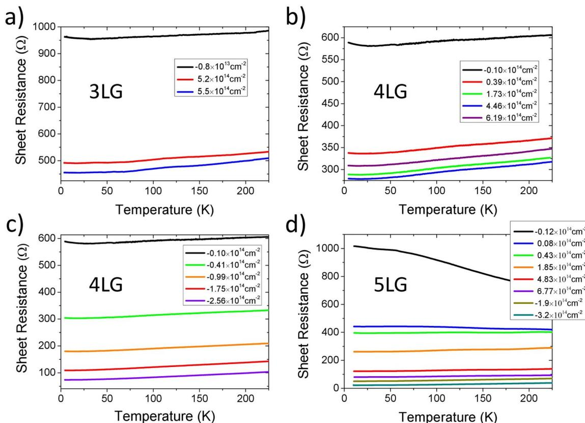
**Figure 3** | The experimental sheet resistances as function of temperature measured at different gating-induced surface charge densities (reported in the legends) in a) a 3LG device for positive gating (electron doping); b) a 4LG device for positive gating; c) the same as in b) but for negative gating (hole doping); d) a 5LG device for positive and negative gating.
