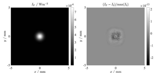
**Fig. 5.** Irradiance (left) and its relative deviation of the directly [ $S_0$  to  $S_2$ , Fig. 2 (top), Test 1 in Tables 1 and 2] propagated linearly  $x$ -polarized Gaussian beam by use of vectorial diffraction integrals from the indirectly propagated one ( $S_0$  via  $S_1$  to  $S_2$ ). The viewing angle is perpendicular to  $S_2$ .
