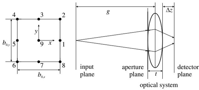
**Fig. 15.** Left: distribution of chosen source points on the input plane for the test of reachability of the detector sampling grid positions of an optical system. The numbering corresponds to the respective source intensity. Right: example of an optical system under test (only marginal rays from a single source point are shown).
