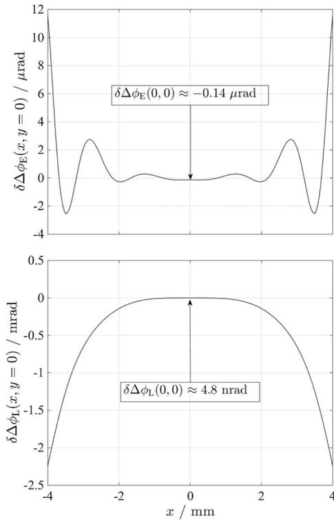
**Fig. 14.** Difference of the phase bias for empty (top) and loaded cavity in the ideal configuration of the interferometer described in [11–13] between the calculation by a vectorial ray-based diffraction integral with spherical wave decomposition (VRBDI-SW) and a vectorial general astigmatic Gaussian beam-tracing algorithm (VGAGB) [13].
