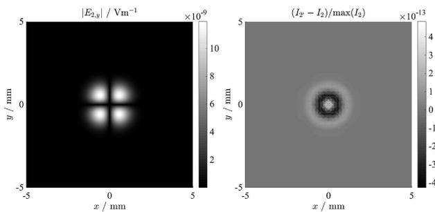
**Fig. 7.** Left: from  $S_0$  via  $S_1$  to  $S_2$  [Fig. 2 (bottom), Test 2 in Tables 1 and 2] propagated  $y$  component of the electric field of a linearly  $x$ -polarized Gaussian beam by use of vectorial diffraction integrals. Right: relative deviation of the irradiance between the directly from  $S_0$  to  $S_2$  and the indirectly ( $S_0$  via  $S_1$  to  $S_2$ ) propagated beam. The viewing angle is perpendicular to  $S_2$ .
