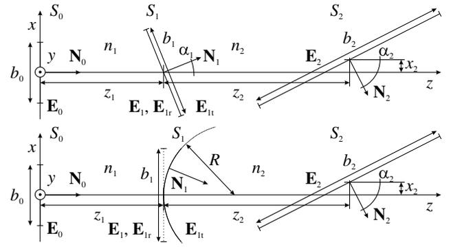
**Fig. 2.** Toy models 1 (top) and 2 (bottom) for the numerical test of power conservation for reflection, refraction, and propagation of electromagnetic fields by vectorial diffraction integrals. An interface separates two transparent, isotropic, homogeneous, and nonmagnetic media with refractive indices  $n_1$  and  $n_2$ . The fixed parameters are listed in Table 1; the variable parameters are given in Table 2.
