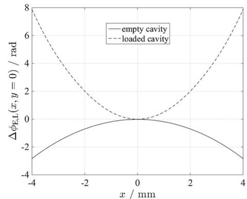
**Fig. 13.** Phase bias for empty and loaded cavity in the ideal configuration of the interferometer described in [11–13] but calculated by the vectorial ray-based diffraction integral with spherical wave decomposition (VRBDI-SW).
