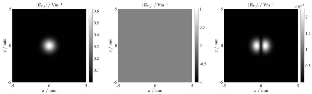
**Fig. 3.** Directly from  $S_0$  to  $S_2$  [Fig. 2 (top), Test 1 in Tables 1 and 2] propagated electric field components of a linearly  $x$ -polarized Gaussian beam by use of vectorial diffraction integrals. The viewing angle is perpendicular to  $S_2$ . The corresponding magnetic components can be found in Appendix C.
