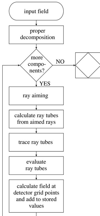
Fig. 9. Flow chart of the VRBDI algorithm.
