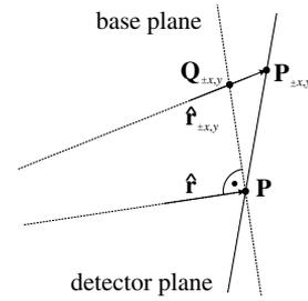
Fig. 19. Situation after ray tracing: the points  $\mathbf{Q}_{\pm x,y}$  on the plane normal to  $\hat{\mathbf{r}}$  have to be found from known intersections  $\mathbf{P}$  and  $\mathbf{P}_{\pm x,y}$  and known versors  $\hat{\mathbf{r}}$  and  $\hat{\mathbf{r}}_{\pm x,y}$ .
