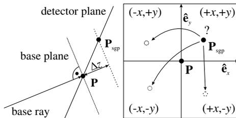
**Fig. 20.** Situation after ray tracing. Left: the intersection  $\mathbf{P}$  of the base ray with the detector plane defines the orthogonal base plane, which does, in general, not contain the nearby sample-grid point  $\mathbf{P}_{\text{sgp}}$ . Further propagation by  $\Delta z$  along the base ray is necessary. Right: the four possible  $\pm$ -combinations of ray vectors are decided by the position of  $\mathbf{P}_{\text{sgp}}$ .
