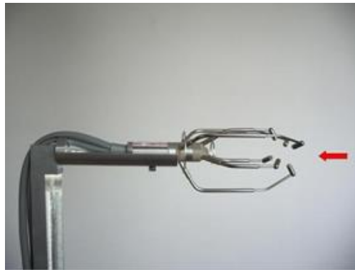
Fig.1. Ultrasonic Anemometer sensing element (the arrow indicates the flow direction)
