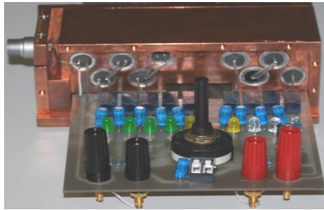
Fig. 2. Photo of the INRIM divider, in which it can be seen the copper box housing the resistors.
