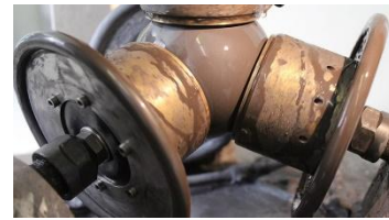
Fig. 28. Lapping tools of the tetrahedron lapping and polishing device designed and used in the PTB manufacturing chain for Avogadro spheres [courtesy PTB].
