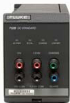
Fig.1. J. Fluke mod. 732 B DC Voltage standard.
