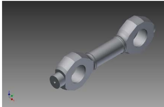
Fig. 1 Structure of the uniaxial force transducer (UFT)
