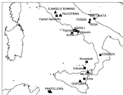
Fig. 6. Location of absolute stations in Southern Italy. Squares represent the reference stations for the relative gravity network, triangles represent the absolute stations located on the dynamic areas. Circles are the stations constituting the fundamental ties of the «Calibration line» for relative gravimeters and a station (Cosenza) settled in a seismic area.
