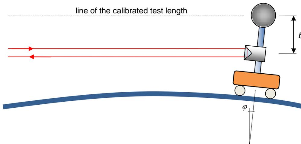
**Figure 2 – Scheme of the Abbe error**
