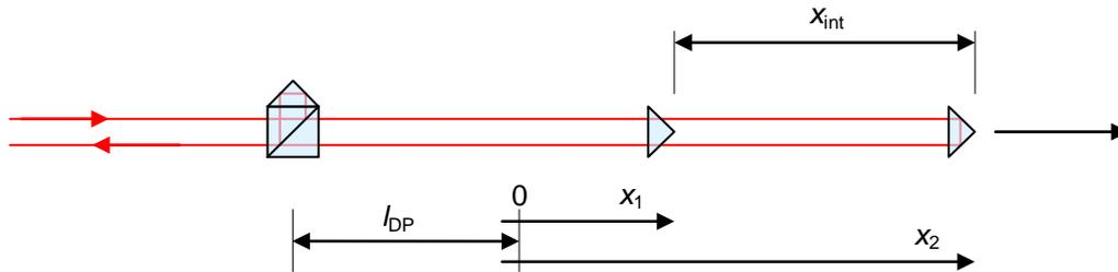
**Figure 1 – Scheme of an interferometric measurement**
