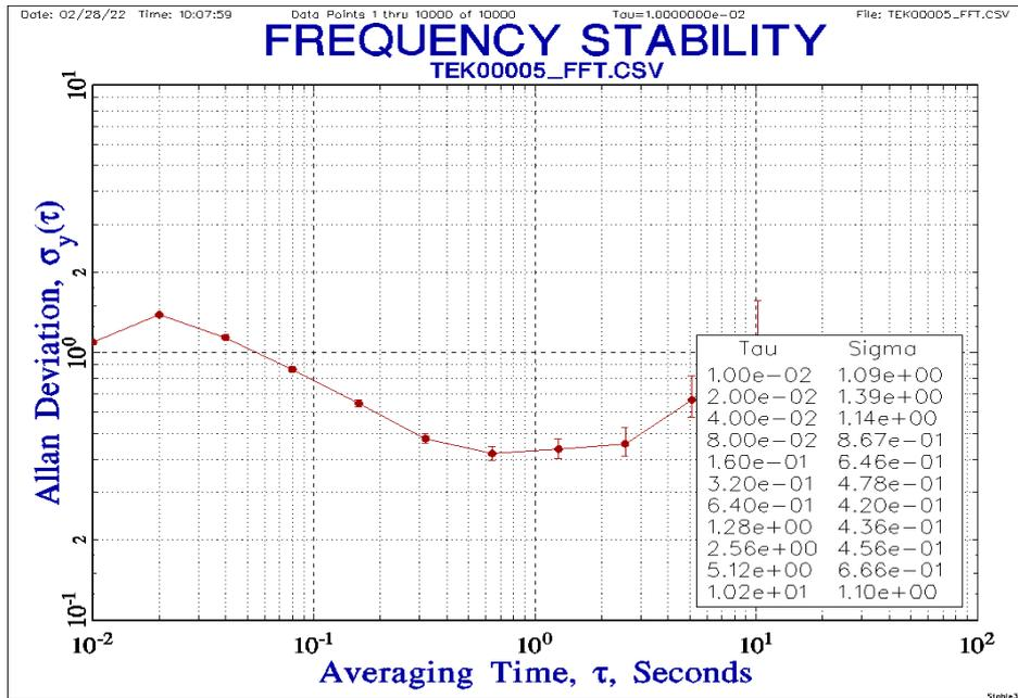
**Figure 9 a).** Allan deviation obtained from the raw data TEK00005\_FFT.
