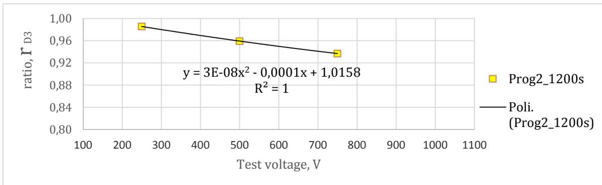
**Figure 29.** The ratio measurements at settle time  $2\tau$  measuring step 3 with autoupdate and its polynomial interpolation. The measurements at 1000 V for the Prog2 are not performed.
