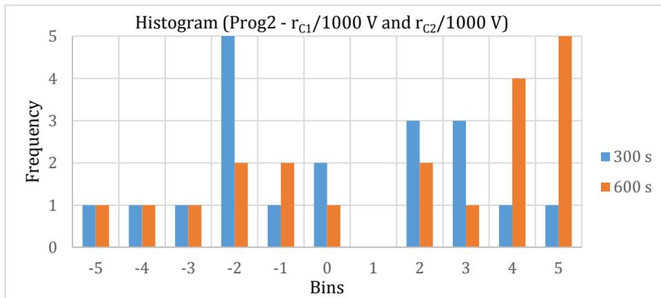
**Figure 25.** The histogram for the program Prog2 at 1000 V for the ratio measurements at settle time of 300 s and 600 s.
