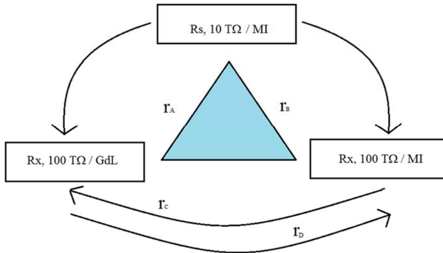
In the case of the comparison D, the value  $r_{D2/1000 \text{ V}}$ ,  $r_{D3/1000 \text{ V}}$  and  $r_{D4/1000 \text{ V}}$ , the measurements at 1000 V for the Prog2, was not performed by the bridge because of the the voltage  $V_s$  on  $S_2$  was out of range and higher than 1050 V, the maximum value supplied by the calibrators. In case of the comparison C at 250 V it was obtained the condition of the equation 5a) but not for the other test voltages.
