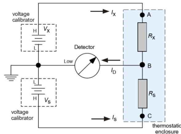
**Figure 1.** The principle of a Wheatstone modified bridge.
