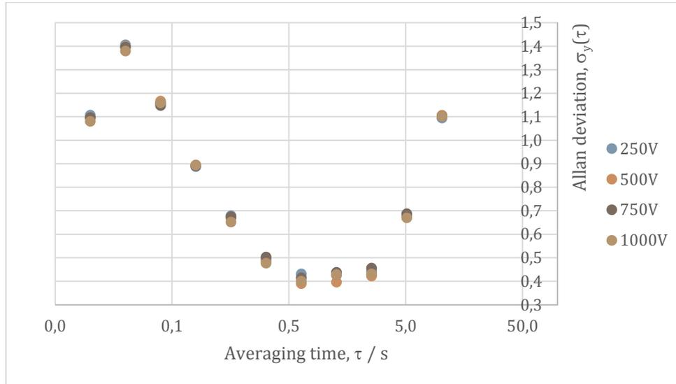
Using Table 6 from the paragraph *Evaluation of the intrinsic noise* of the dc sources, we can obtain for the white noise regime the relationship between the Allan deviation and the standard deviation. The result are reported in table 2.
