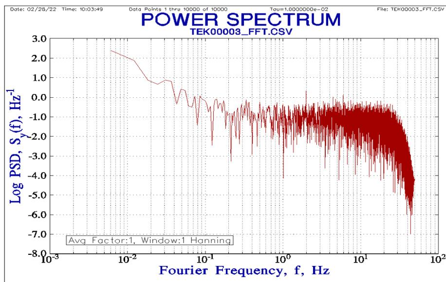
**Figure 8 a).** PSD obtained for the first comparison at positive polarity of  $R_x$  ( $R_s$ , 10 T $\Omega$  / MI :  $R_x$ , 100 T $\Omega$  / GdL) and test voltage of 1000 V, in the frequency range from 0 Hz to 50 Hz.
