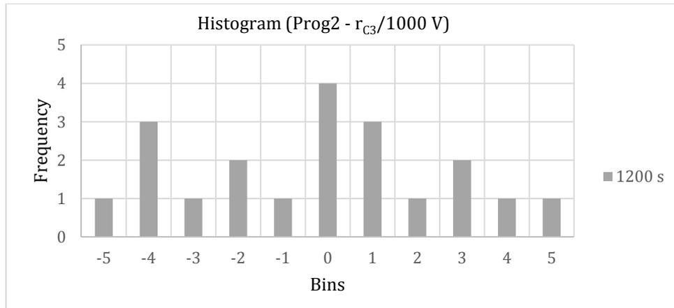
**Figure 26.** The histogram for the program Prog2 at 1000 V for the ratio measurements at settle time of 1200 s / step 3.
