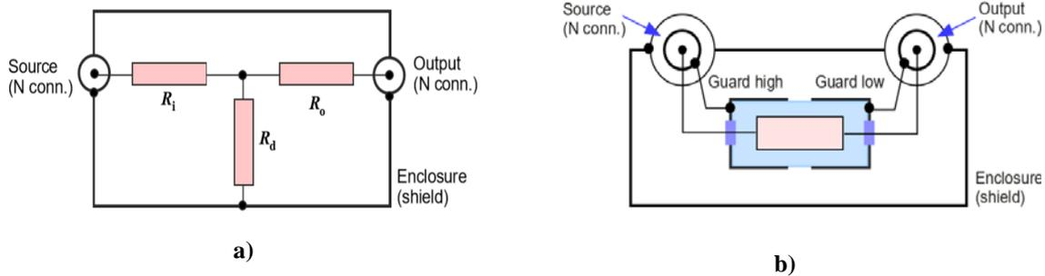
**Figure 2.** Representation of the high value resistors. The shield delimits the electrical resistance inside and outside the ports Source and Output. a) network resistors b) unique resistive element.
