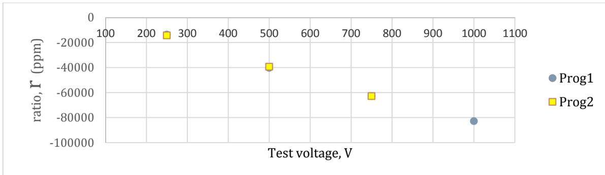
**Figure 28.** Relative deviation of the measurements at settle time  $3\tau$  measuring at constant settle time (blue dots) in Prog1 and with autoupdate (yellow dots) in Prog2. (the uncertainties are less than the dots and it can't be shown). The measurements at 1000 V for the Prog2 was not performed by the bridge.
