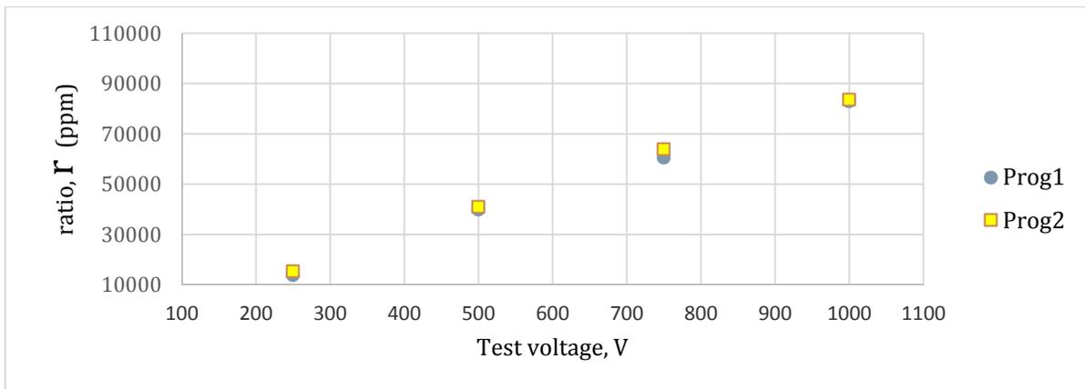
**Figure 22.** Relative deviation of the measurements at settle time  $3\tau$  measuring at constant settle time (blue dots) in Prog1 and with autoupdate (yellow dots) in Prog2. (the uncertainties are less than the dots and it can't be shown).
