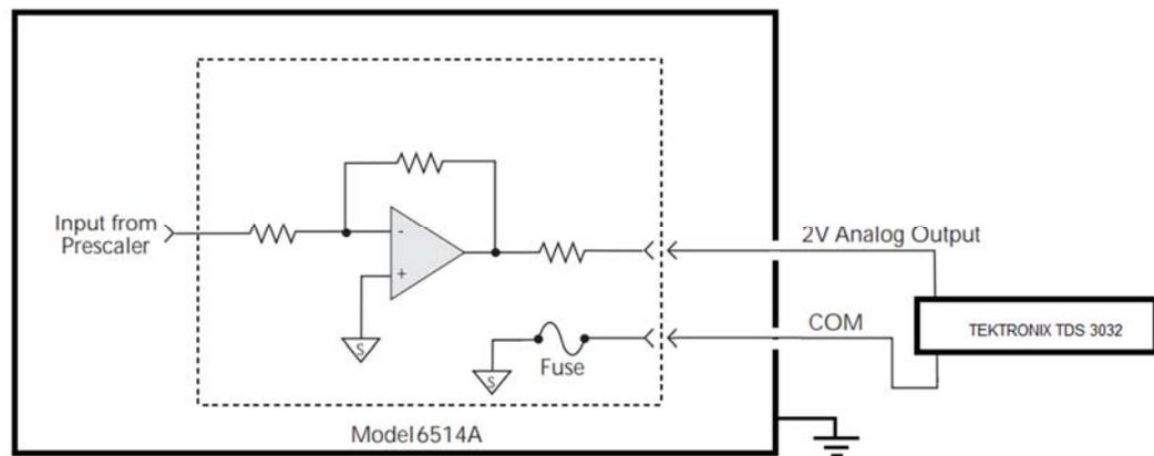
**Figure 7.** Output circuit to 2 V connection at the voltage input of the oscilloscope Tektronix, model TDS 3032. The bold line indicates the shielded room of the laboratory, connected to the ground potential.
