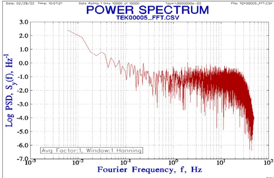
**Figure 8 b).** PSD obtained for the first comparison at negative polarity ( $R_s$ , 10 T $\Omega$  / MI :  $R_x$ , 100 T $\Omega$  / GdL) and test voltage of 1000 V, in the frequency range from 0 Hz to 50 Hz.
