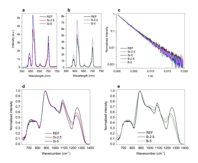
**Fig. 3**. (A,B) Luminescence intensity of the samples with addition of  $SiO_2$  (a) and  $B_2O_3$  (b) in relation to the REF sample. The excitation is at 395 nm. (c) Luminescence decay curves of the  $Eu^{3+}$ -doped glasses excited at 395 nm and monitored at 612 nm. (d,e) Normalized IR spectra of the glasses with varying  $SiO_2$  (d) and  $B_2O_3$  concentration (e).
