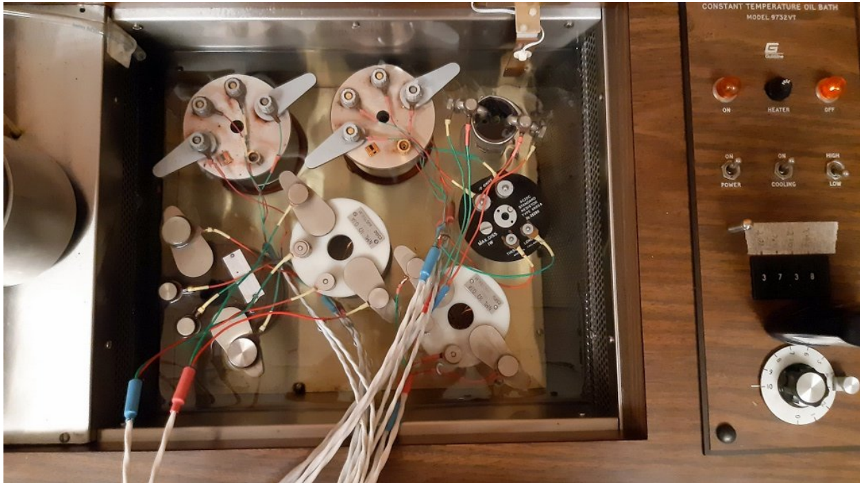
Fig. 2 - Guildline 9732 VT oil bath. The short-term stability of the bath is approximately 0.001°C
