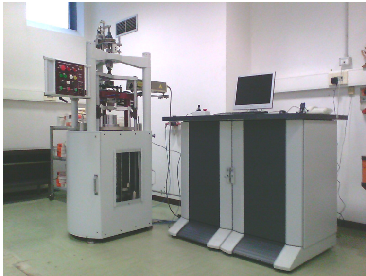
Figure 2: Primary Hardness Standard Machine at INRiM
