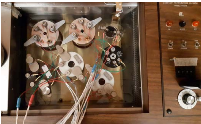
Fig. 2a. Guildline 9732 VT oil bath. The short-term stability of the bath is approximately 0.001°C.
