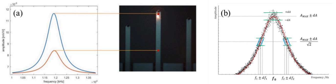
Fig. 7. (a) Experimental values of the cantilever resonance peaks (fitted by Lorentzian functions), determined at different positions along the cantilever; (b) method applied for quality factor estimation (from experimental data).
