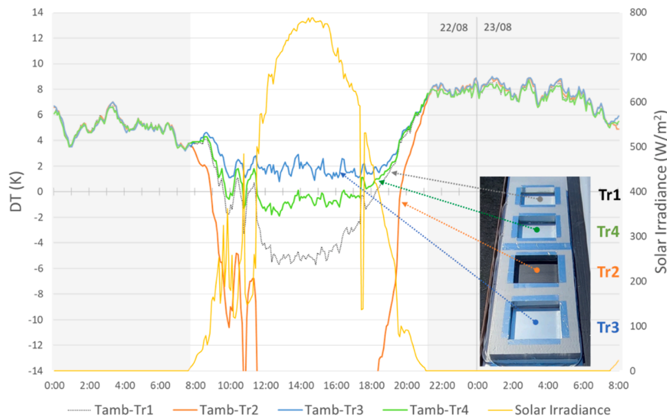
Fig. 3. Difference between ambient air temperature and reference temperatures Tr1–Tr4 along with the irradiance. Data for 22–23 Aug 2024. Tr1: 1 mm steel sheet, painted white. Tr2: polypropylene panel sample. Tr3: polypropylene panel sample coated with SSF material. Tr4: 1 mm aluminum sheet coated with SSF material.
