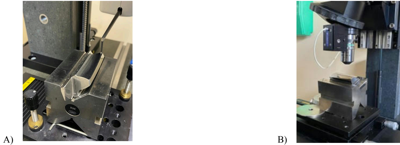
Figure 33: A) Gear 825 measured by stylus profilometer, B) Gear 825 measured by stylus profilometer.
