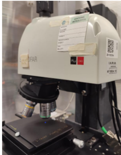
Figure 2: SENSOFAR PL \mu 2300 optical profilometer.
