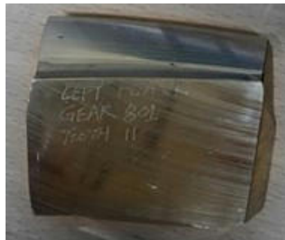
Figure 7: Gear tooth 801 produced by Newcastle University.
