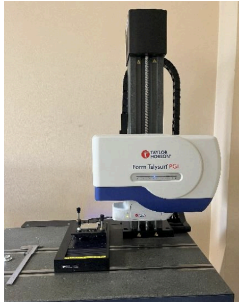
Figure 1: TAYLOR HOBSON FORM TALYSURF PGI NOVUS S10 stylus profilometer.
