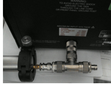
Fig. 1. Short connection of the TVC to the JAWS inside the pulse-tube cryocooler through the vacuum-tight SMA feedthrough.
