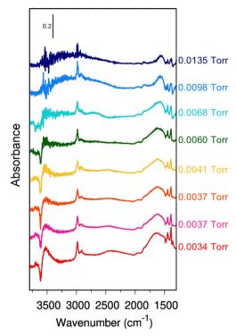
Fig. 2 Incremental variation of absorbance with pressure (dA). Increasing pressure from red to blue – see Fig. 1, panel A. On the right side, we report the equilibrium pressure at which each spectrum has been measured. The spectra are all reported in arbitrary units. No baseline correction has been introduced
