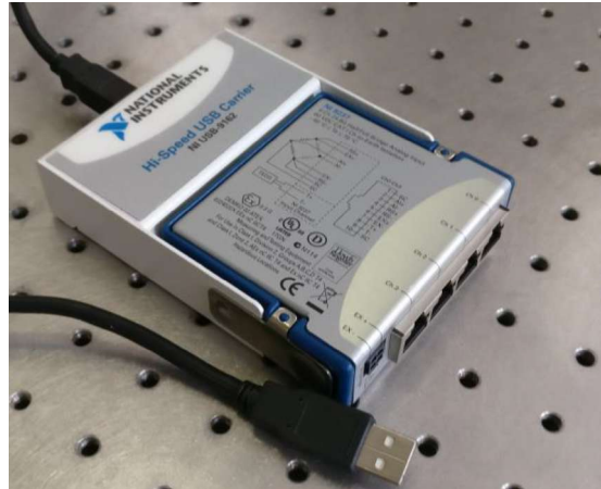
Fig. 2. NI-9237 measuring amplifier [8].
