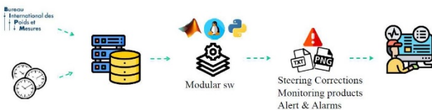
Fig. 4. Modular software architecture for the generation of UTC(IT)
