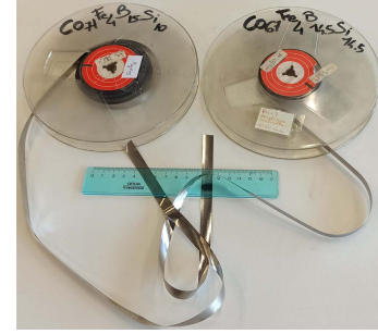
Fig. 1. Ribbons of \text{Co}_{67}\text{Fe}_4\text{B}_{14.5}\text{Si}_{14.5} (right) and \text{Co}_{71}\text{Fe}_4\text{B}_{15}\text{Si}_{10} (left) composing core 1 and 2, respectively.
