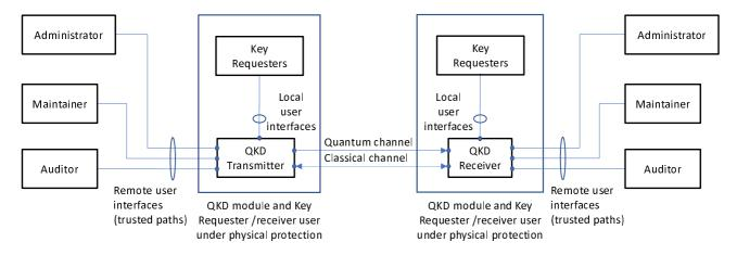
Figure A.6: Example layout of QKD modules, TOE users and physically protected areas
