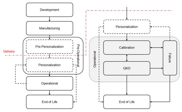
NOTE: (Left) Complete life-cycle. (Right) Close-up of post-delivery phases, including operational states of the TOE. Individual dashed elements can be empty and are not defined in this PP.
