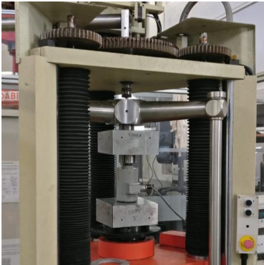
Figure 1: The 20 kN transducer placed between the 3° tilted plates integrated into the MCF30 FSM
