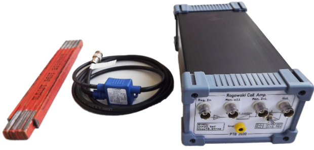
Fig. 7: Rogowski coils with the corresponding electronic integrator.
