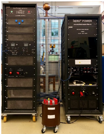
Fig. 3: Two power amplifiers and a current generation transformer with several rated current ranges from 5 A to 200 A.
