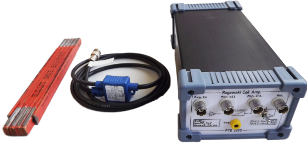
Fig. 7: Rogowski coils with the corresponding electronic integrator.
