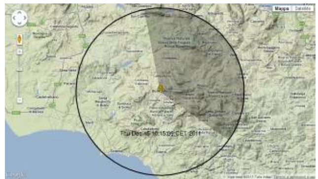
Fig. 3. Map example (no rain) projected over a cartographic system provided by Google©. The image refers to the radar installed in Bisacquino (PA). The gray area is the graphical representation of a blanked region.
