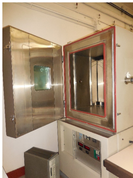
Figure 2. Climatic chamber Weiss Technik in operation at INRiM and used, coupled with the Kambic chamber, to test RS92 and RS41 before and after fast temperature changes.
