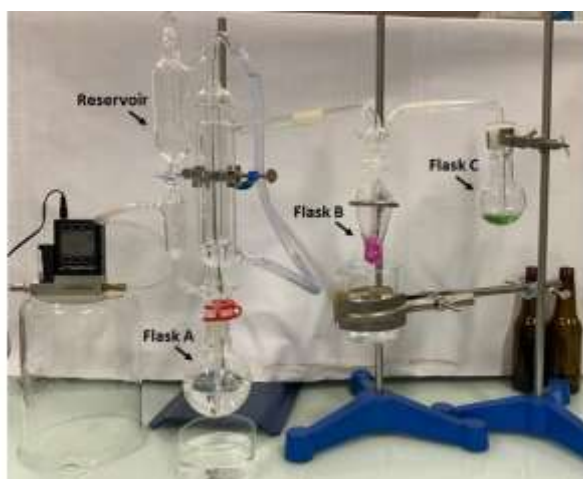
Figure 1: INRiM measurement system for the extraction phase of the determination of free \text{SO}_2 by 591A method
