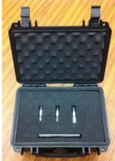
Figure 4: Shipping container with three indenters
