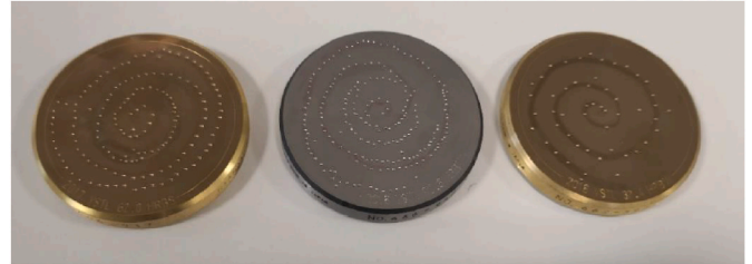
Fig. 2. The blocks used for Rockwell B hardness tests. The indentations derived from the hardness tests are visible. The distances between the centres of two adjacent indentations fulfil the requirement of the standard. Additional indentations are subsequently carried out to settle the blocks and the indenter.
