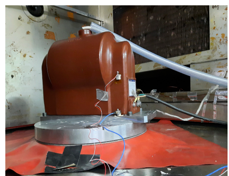
Figure 2. Assessing VT frequency response under temperature and vibration. (a) Scheme of the measuring system; (b) overview of the whole setup arranged at LNE; (c) detail of the generator and the voltage standard transformer, (d) DUT mounted onto the shaker inside the temperature chamber.
