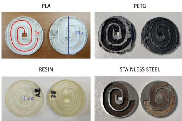
Figure 1 3D-printed prototypes in FDM-PLA, FDM-PETg, SLA-Resin and SLM-Stainless Steel, cut in half to show the upper (left) and lower (right) faces.
