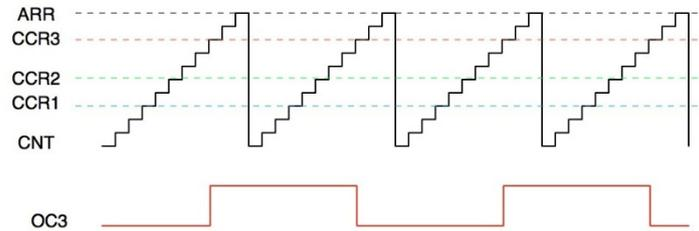
This allows to have a fixed frequency square wave output, which can be calculated based on the clock frequency, the prescaler and the *ARR* (auto reload register) value.
