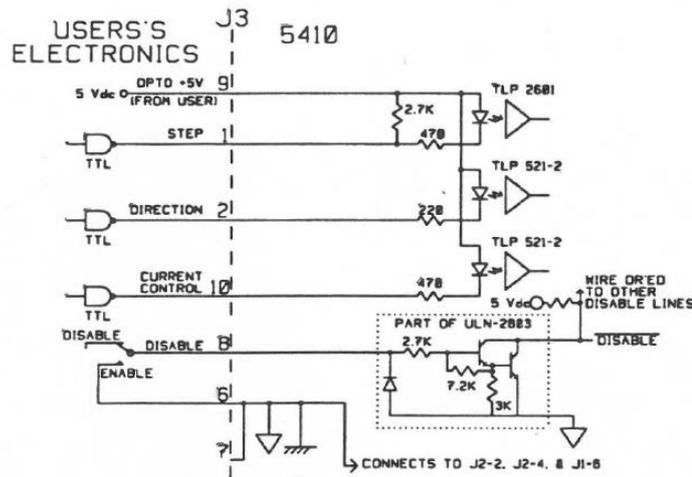
The driver accepts TTL signals at its input, the microcontroller has outputs in CMOS logic (3.3V) 5V tolerant, the enable and direction pins have therefore been configured as open-collector outputs, inserting a pull-up resistor to move the output characteristic between 0 V and 5 V.
