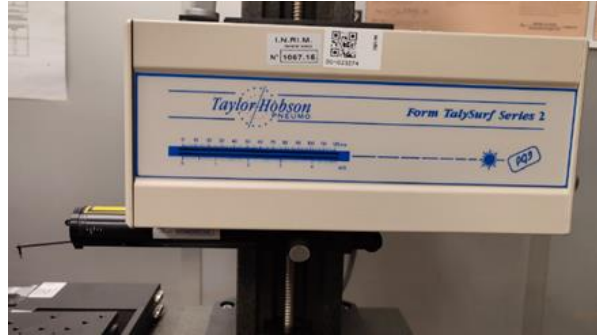
FIGURE 2 - TAYLOR HOBSON TALYSURF SERIES II STYLUS PROFILOMETER
