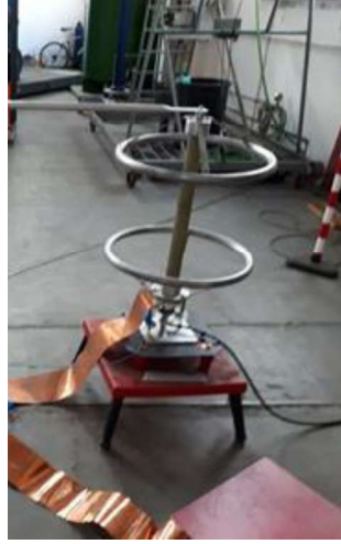
Fig. 1. SAGI 304 resistive divider up to 200 kV.
