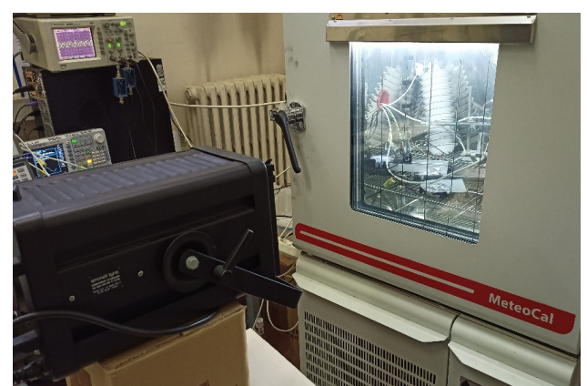
Figure 7. (a): Scheme of the set-up to check for the effect of irradiation where the lamp (L) is moved in different positions in front of the window. The marks T in the picture indicate the three naked Pt100, while the mark R stands for the radiation-shielded Pt100. The red circles represent the transmitter and the receiver of CAT. (b): A picture of the setup where the 1000 W halogen projector is visible in the foreground. On the right, the climatic chamber where the CAT and the thermometers are visible through the window.
