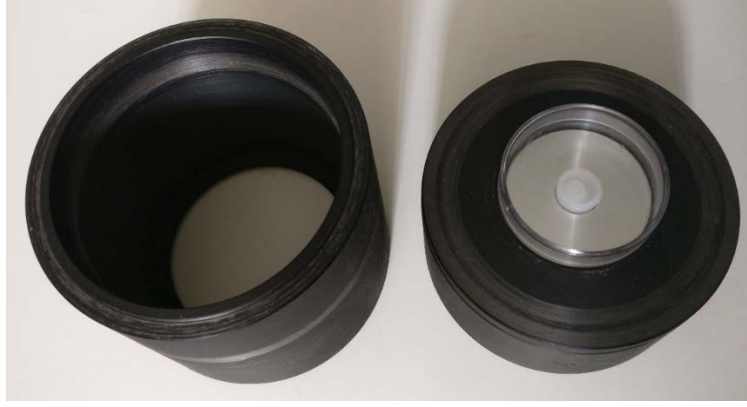
Figure 10: Counting spacers for d_{80} (left) and d_{40} (right) nominal positions. The gamma counting container with the cut 3 mL PE vial centered by the hollow disk is visible on top of the d_{40} spacer.
