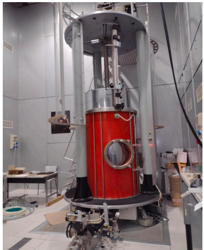
Fig. 2. Large piston prover at INRIM, typical configuration.
