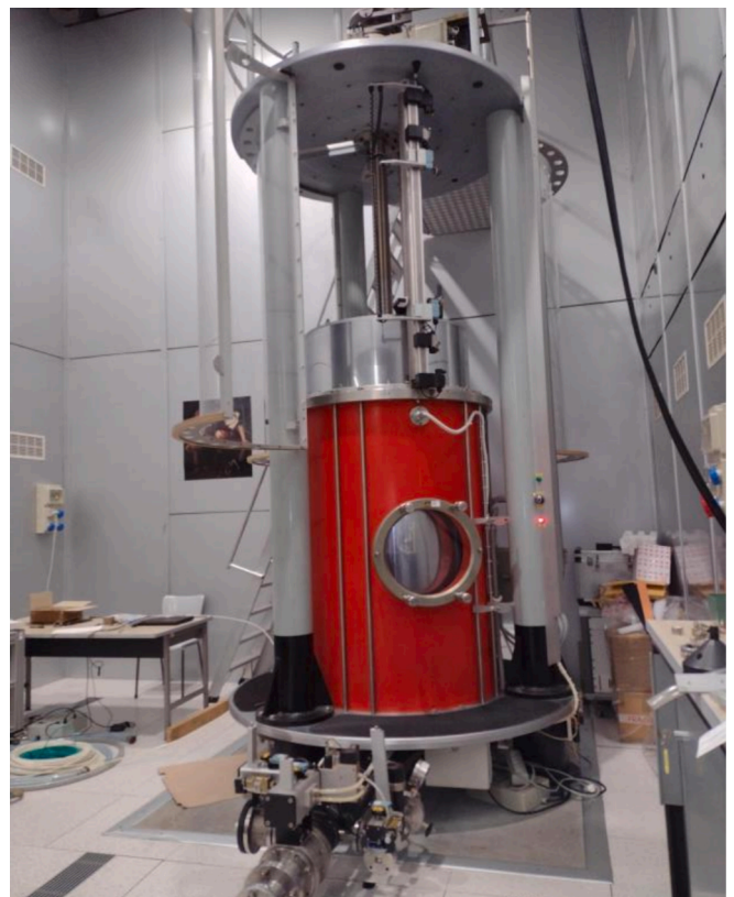
Fig. 2. Large piston prover at INRIM, typical configuration.
