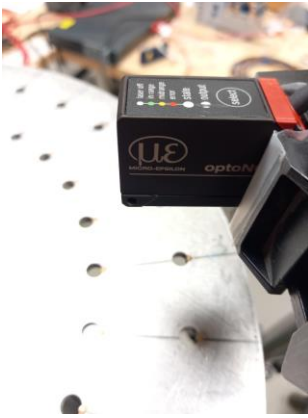
Fig. 3 Displacement sensor for the characterization of the test bench.
